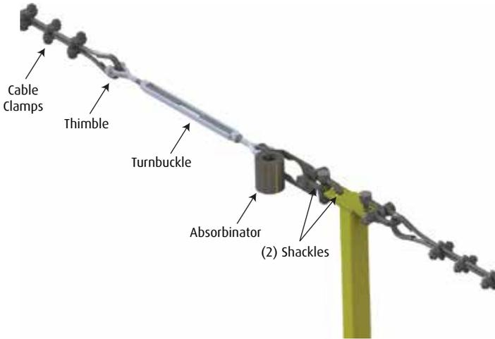
4. For all Absorbinators, attach Absorbator to steel shackle or compatible carabiner, attach shackle/carabiner to second shackle, and attach second shackle to Stingray Anchor connection point. For all shackles, tighten bolt until at least one thread is fully visible.
