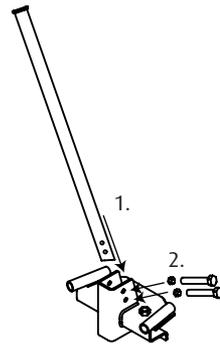
4. Place Stingray Anchor at selected installation location on structural beam. Tilt Base Assembly to one side and tighten Mounting Bolt on that side until snug. Repeat for opposite side. Ensure back of Base Assembly throat is flush against beam flange.
